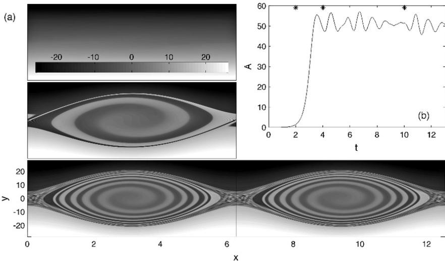
**Figure 13.7.** Evolution of the single-wave model [BAL 13]. a) Plot of a typical phase space hole pattern. b) Behavior of mode amplitude as a function of time
