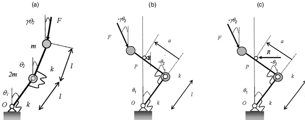
Fig. 1. Ziegler's pendulum under partial follower load: (a) free system and (b, c) kinematically constrained system. (b) Meaning of the constraint: a sliding support. (c) Equivalent forces: horizontal reaction.
